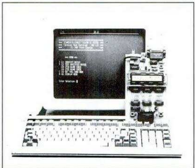
Photo 1: The Circuit Cellar IC tester shown here is operating in terminal mode, connected to a Tandy DT-100 terminal via the RS-232C port on the top of the tester.
