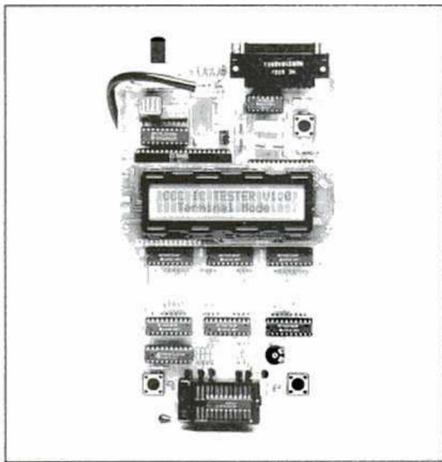
Photo 2: You can use the IC tester in stand-alone mode, provided you have attached the tester's optional LCD. The push-button switches in the upper right, lower left, and lower right control the tester's operation.
