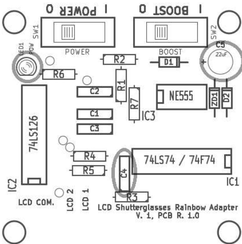
**Electrolytic Capacitors and LED: 4.7 $\mu$ F x1 (C4), 22 $\mu$ F x1 (C5), 3mm LED x1 (LED1)**
