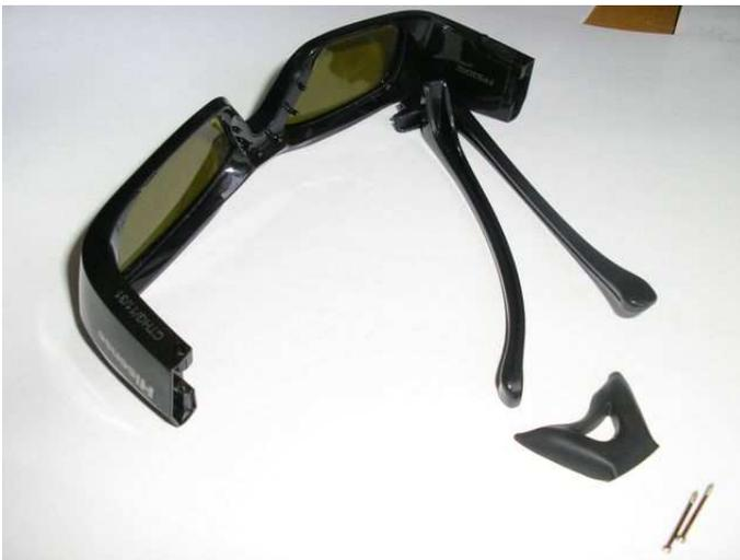
Next the plastic clips that hold the glasses together will have to be prised apart. Use a flat head screwdriver to slip into the gap and lever the front apart from the back. The strength of the clips can vary and it may be impossible to separate the halves without damaging the plastic, but try hard to avoid putting pressure on the glass it can easily crack.
