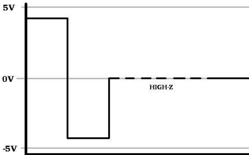
**Figure 2, Output Waveform.** Shows voltage measured over LCD COM. and either LCD 1 or LCD 2 output, with no LCD element connected. Begins at the rising edge of the clock cycle. The dotted line indicates that both output buffers on the LCD output are in 3-State mode.
